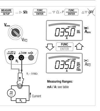
5.9.4 Alternating Current Measurement with Clip-On Current Sensor, A AC and Hz  $\,$
