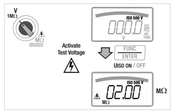
Auto-ranging is active during insulation resistance measurement.
